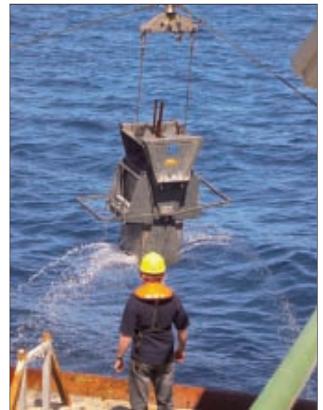
Samples of seabed sediments are collected by box corer.
